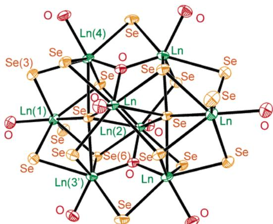
**Figure 1.** ORTEP diagram of the  $(\text{THF})_8\text{Ln}_8\text{Se}_2\text{O}_2(\text{SePh})_{16}$  core, with the C and H atoms removed for clarity. Labeled atoms are mentioned in the text. Primed atoms are related to unprimed ones by inversion symmetry.
