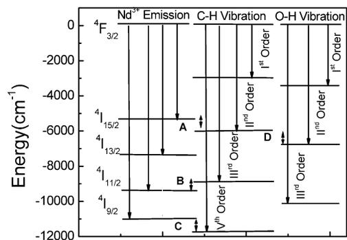
**Figure 4.** Schematic representation of the vibrational quenching of the  ${}^4F_{3/2}$  emission in  $Nd^{3+}$  by the vibrational modes of CH and OH functional groups. The energy differences between the interacting levels of  $Nd^{3+}$  and the vibrational groups are labeled with A, B, C, and D where  $\Delta E_A = 489\text{ cm}^{-1}$ ,  $\Delta E_B = 435\text{ cm}^{-1}$ ,  $\Delta E_C = 565\text{ cm}^{-1}$ , and  $\Delta E_D = 1432\text{ cm}^{-1}$ .
